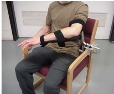
Figure: MKI sleeve and MAST devices: Sleeve array of Force-Sensitive resistors wearable on forearm; Arm support device for extension about the elbow.
